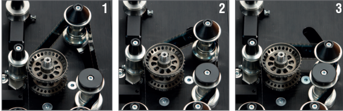
Film transport adjustment for shrunken material: variable film contact with sprocket roll (1: minimum, 2: medium, 3: maximum contact)
