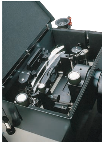
Film Run Mechanism for 35 mm / 8 perf
